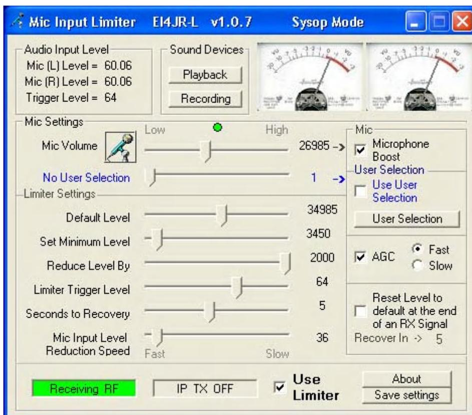
The Mic Input Limiter is a simple to use Windows XP utility that allows the Sysop of a Repeater / Link or PC User to try and control the audio going into their node / link. It cuts down the mic gain when strong audio is used.
